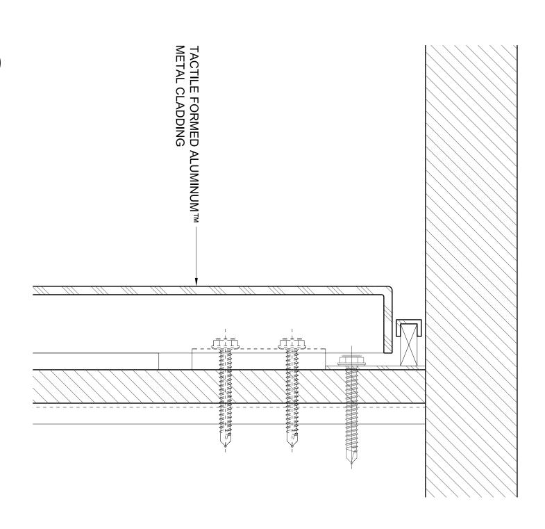
Section - Parapet Return Detail - Tactile Formed Aluminum™ Metal Cladding
