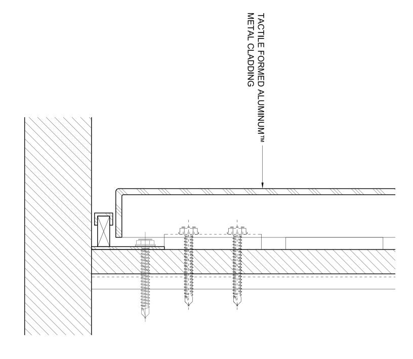
Section - Sill Detail - Tactile Formed Aluminum™ Metal Cladding
